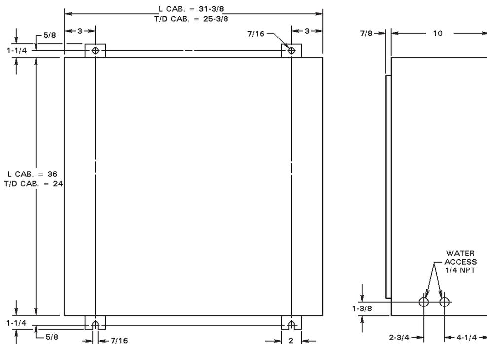
Figure 5-11. "T/D" and "L" Cabinets mounting
