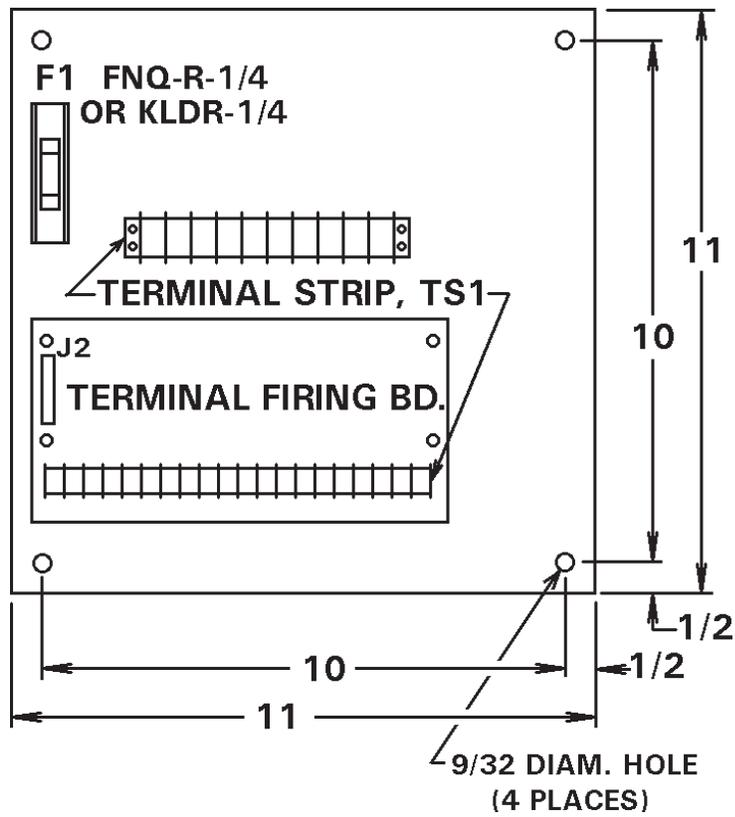
**Figure 5-4.** *11x11 Flat Plate Installation*
