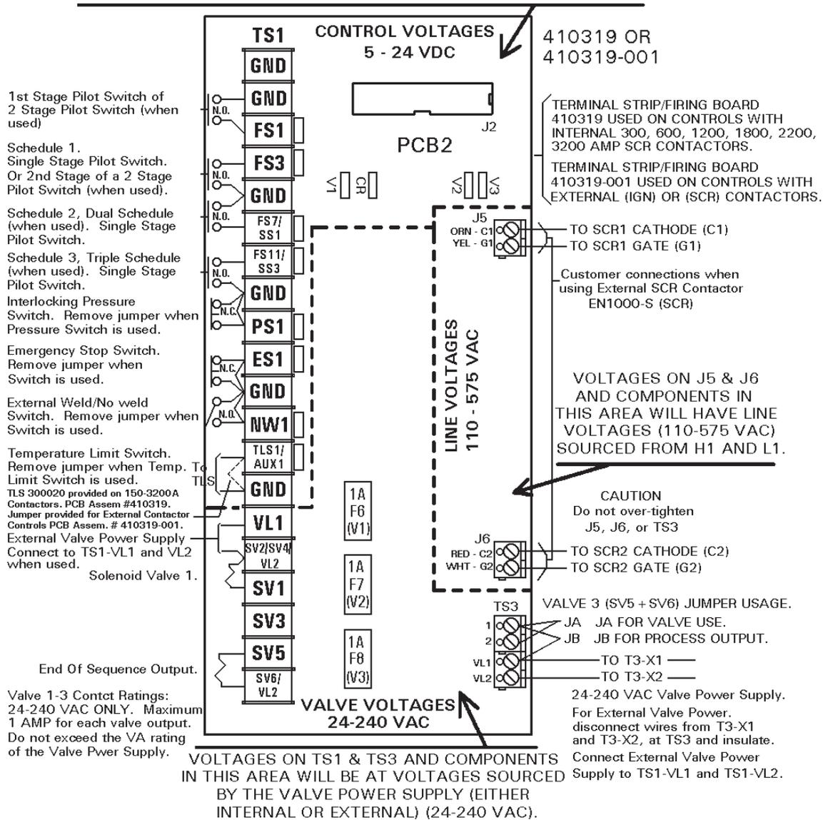
Figure 5-1. Terminal Strip/Firing Board (before June 2004)
