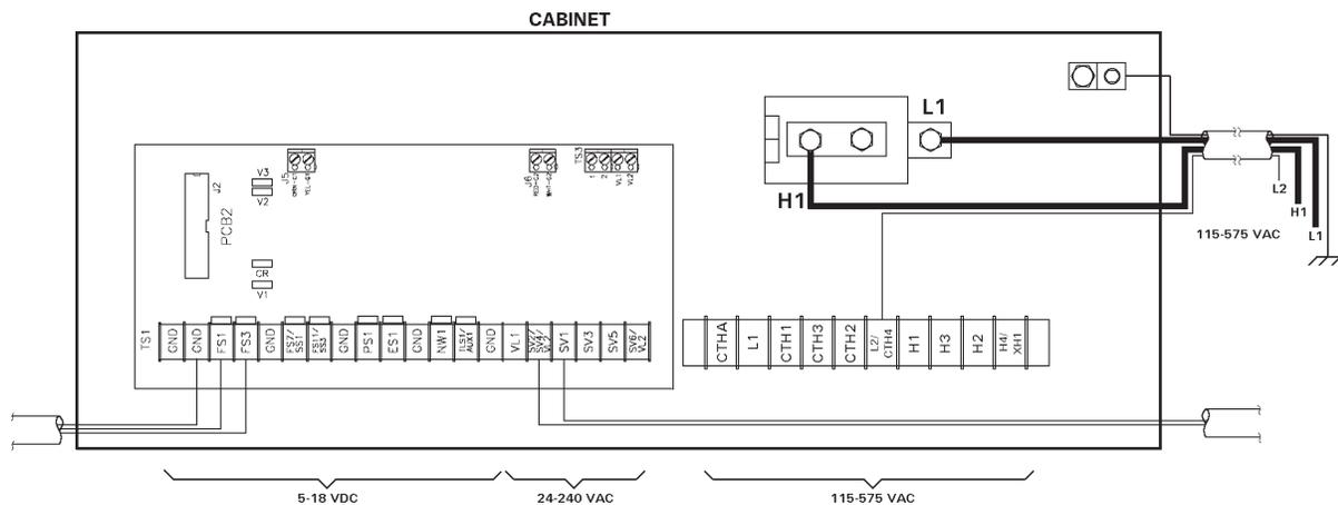
**Figure 4-1.** Recommended low and high voltages conduit wiring and routing
