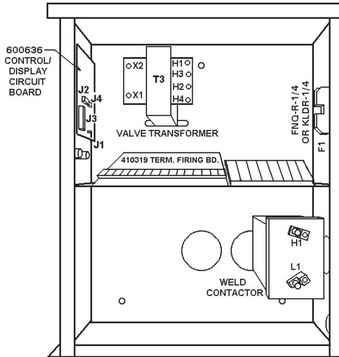
**Figure 5-6.** "E" Cabinet – 300/600/1200A Contactor
