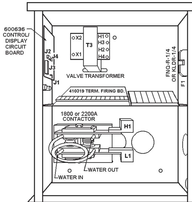
**Figure 5-7.** "E" Cabinet – 1800/2200A Contactor
