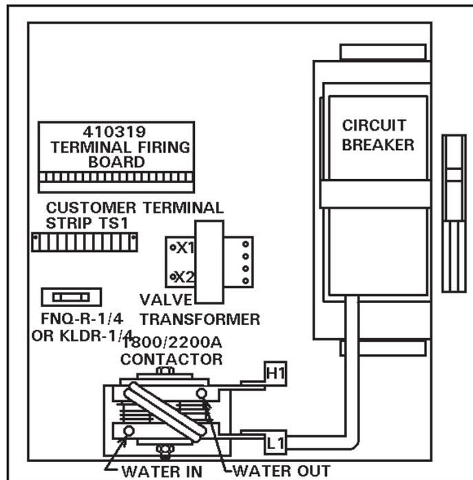
Figure 5-9. “T/D” and “L” Cabinets – 1800/2200A Contactor
