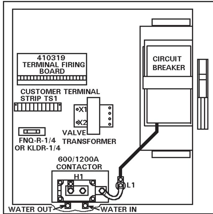
Figure 5-8. “T/D” and “L” Cabinets – 600/1200A Contactor
