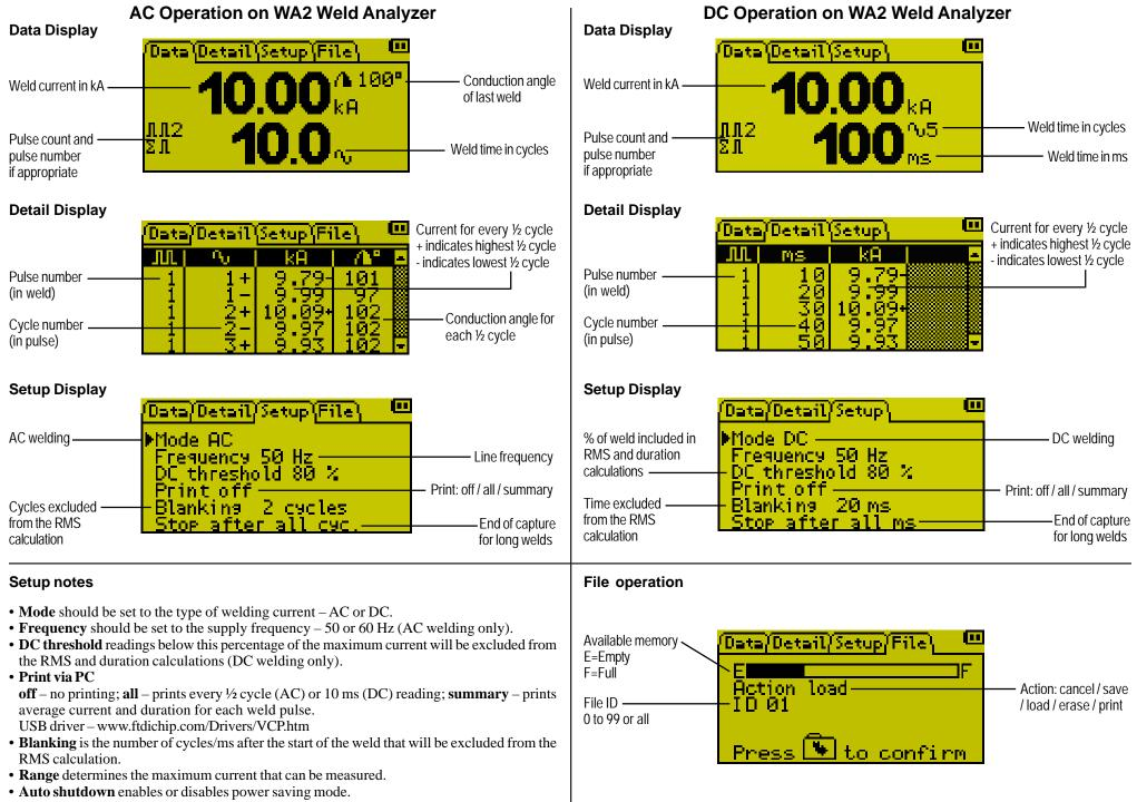
• Stop after nn cycles/ms can be used to capture a specific section of a long weld. If the weld is longer than this parameter, a symbol will be shown alongside the weld time.
