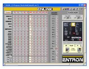
A PC or Laptop with RS232/RS485 converter and ENLINK 1000/1001 for Windows may be used as a master device to communicate with EN1000 Series Controls.
