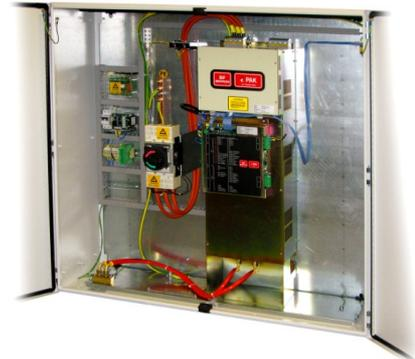
Complete engineered welding control in self contained easy to install cabinet, including safety screens, circuit breaker with door interlocking, optional isolation contactor, power supplies and earth leakage protection.
