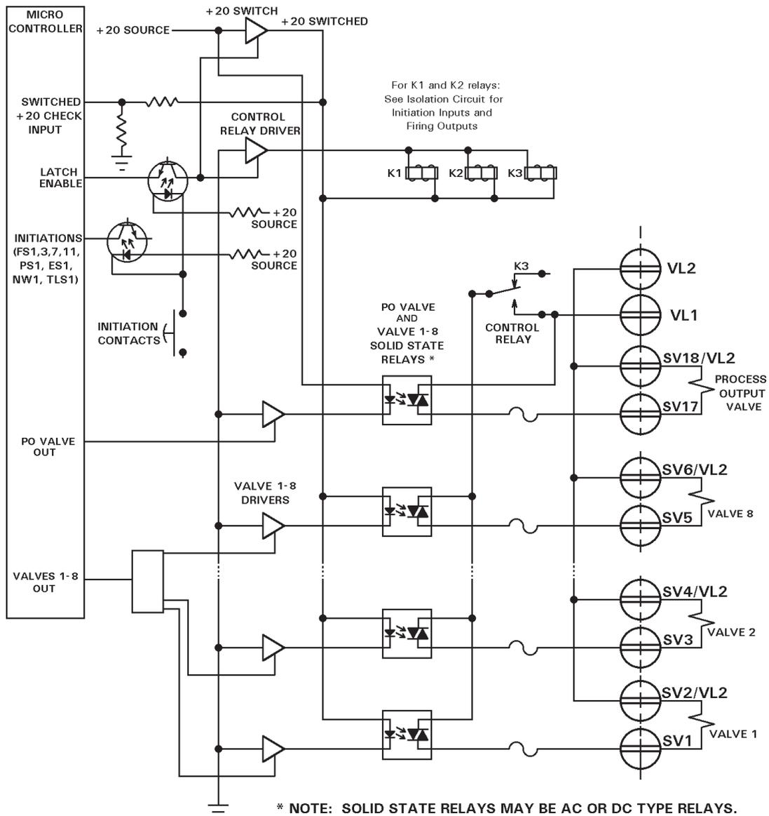
Figure 4-15. Isolation circuit block diagram for valve outputs
