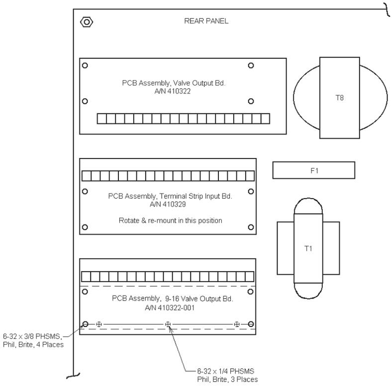
**Figure D6. 9-16 Valve Extension Mounting detail
