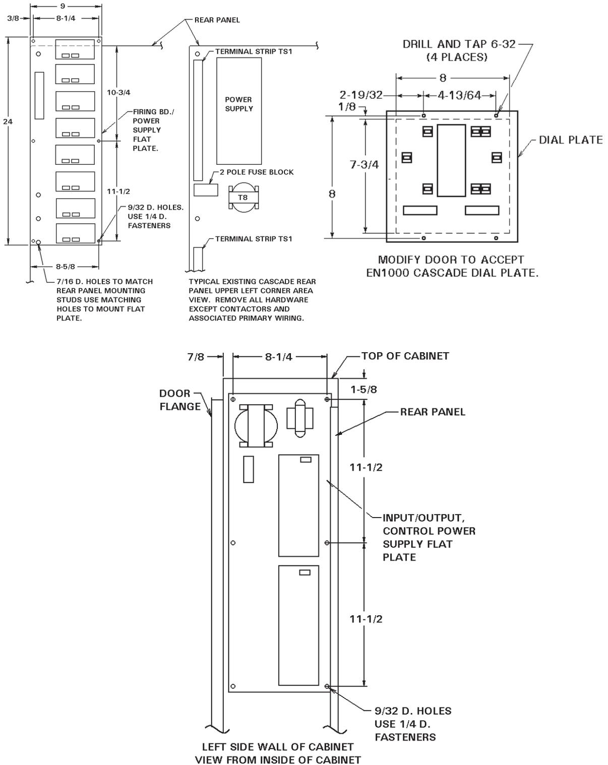
**Figure 3-6.** *Mounting information for Flat Plate Control in existing enclosure*
