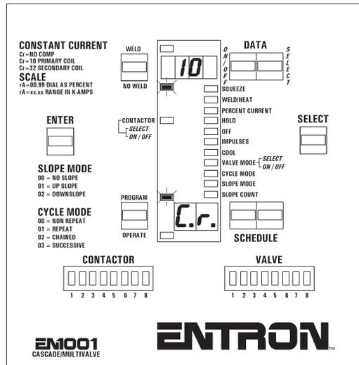
Figure B24. For Primary Coil Sensing
