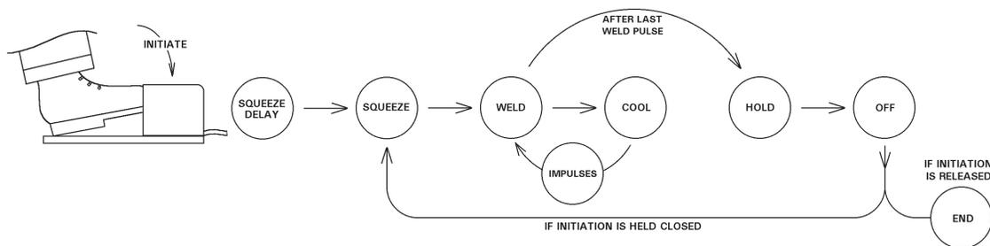
**Figure 9-10.** *SQUEEZE DELAY operation*
