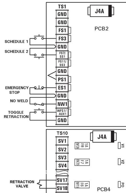
Figure 9-12. Maintained Closure Retraction connections
