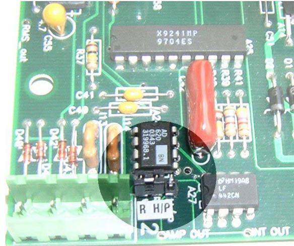
**Figure 8-5.** Jumper setting:
