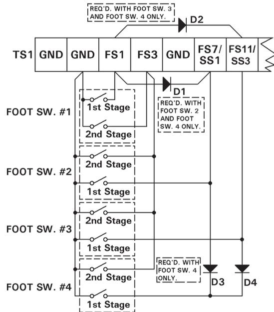
**Figure 5-12. Multiple two-stage foot switch initiation**
