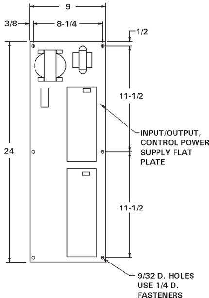
**Figure 3-3.** *Input/Output Assembly mounting detail*
