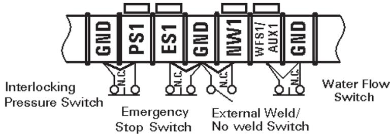
**Figure 4-9.** Other inputs on Terminal Strip TS1
