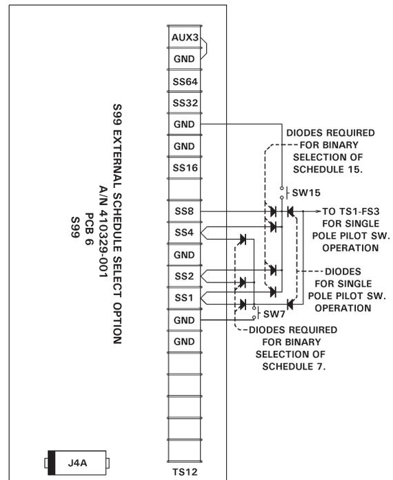
**Figure 5-16.** Multiple pilot switch connections
