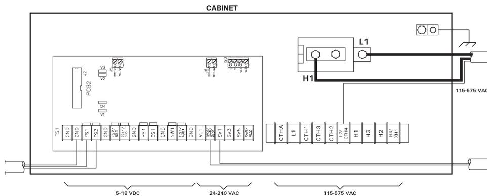
**Figure 4-13. Recommended routing of low and high voltage wires**
