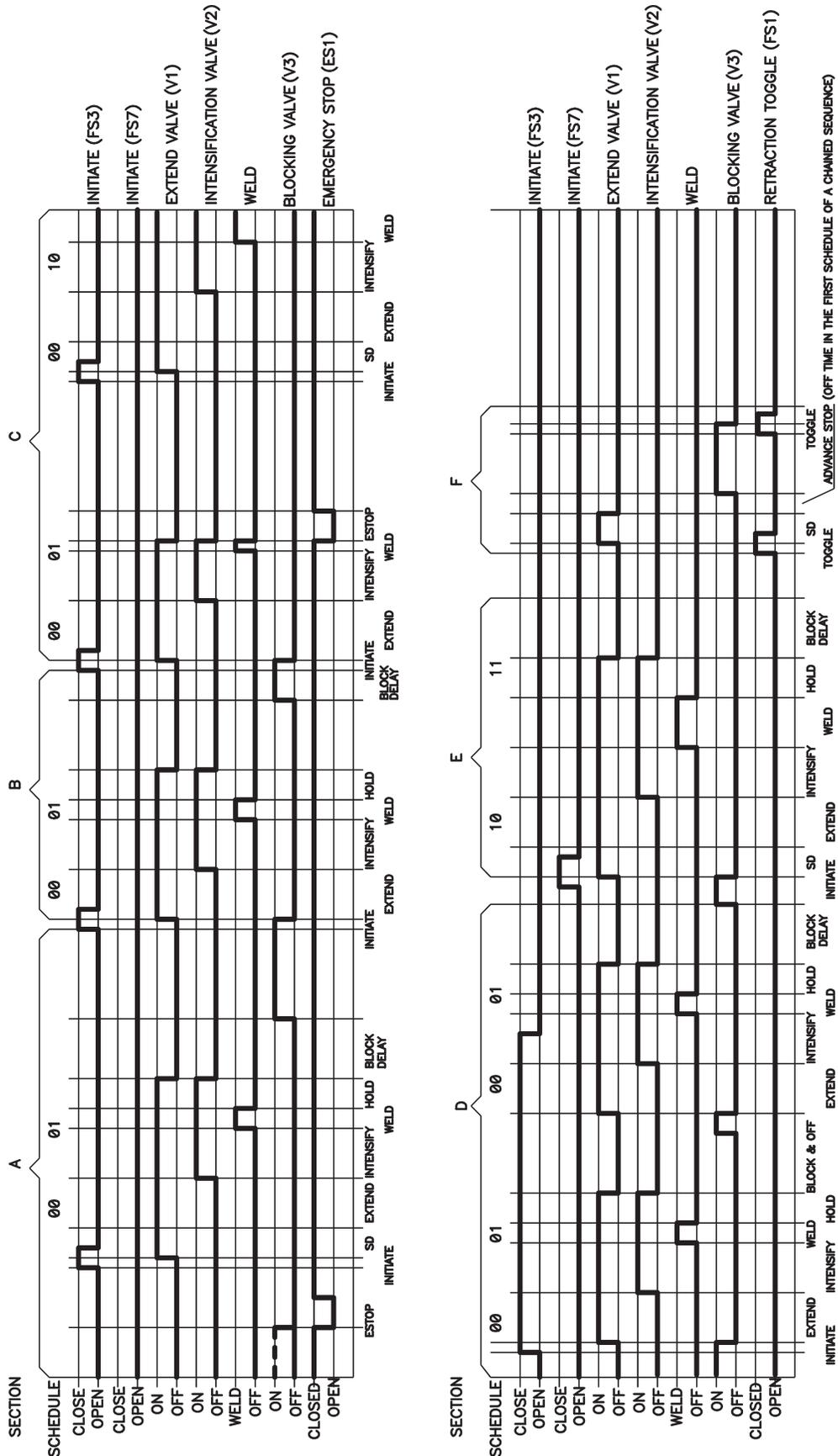
Figure 9-14. Air Over Oil Retraction timing diagrams
