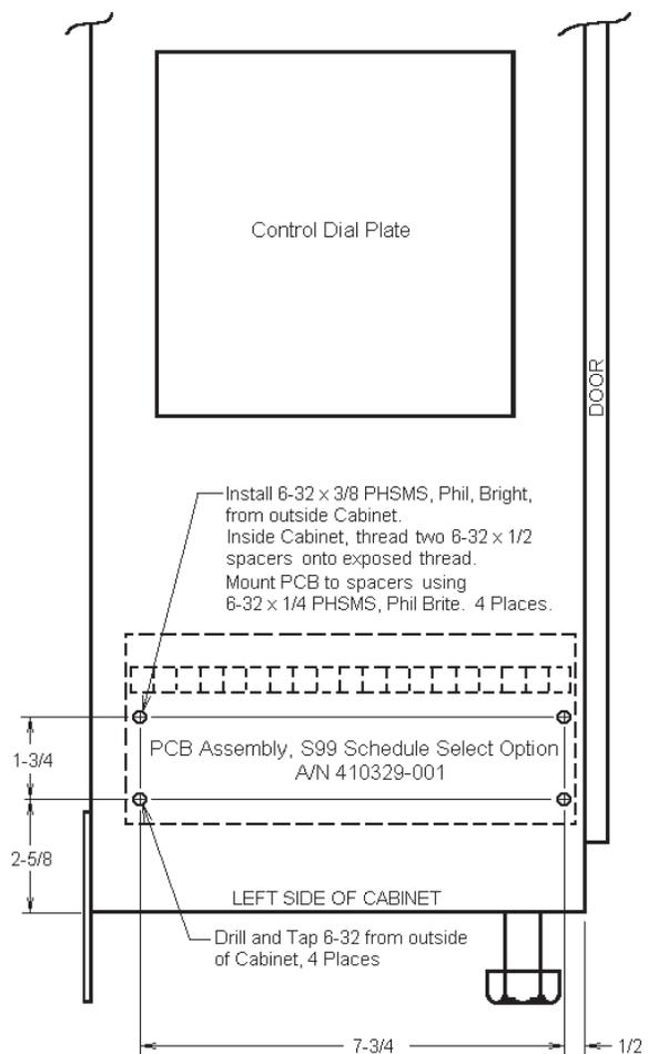
**Figure C2. Mounting detail for
