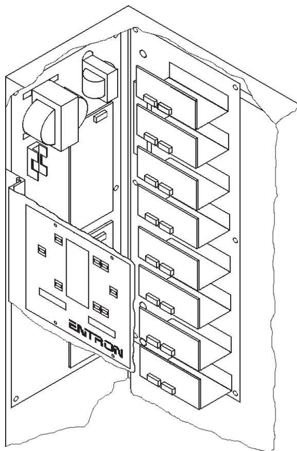
**Figure 3-5.** *Control Panel placement in existing enclosure*
