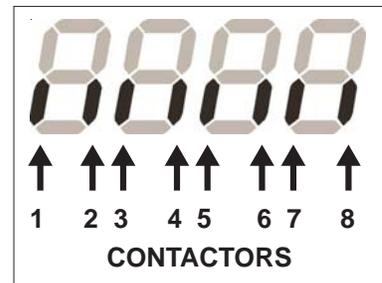
**Figure 5-10.** Contactor indication in DATA display
