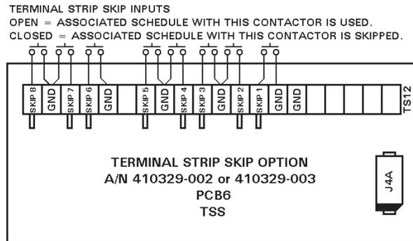
Figure E1. TSS Circuit Board connections
