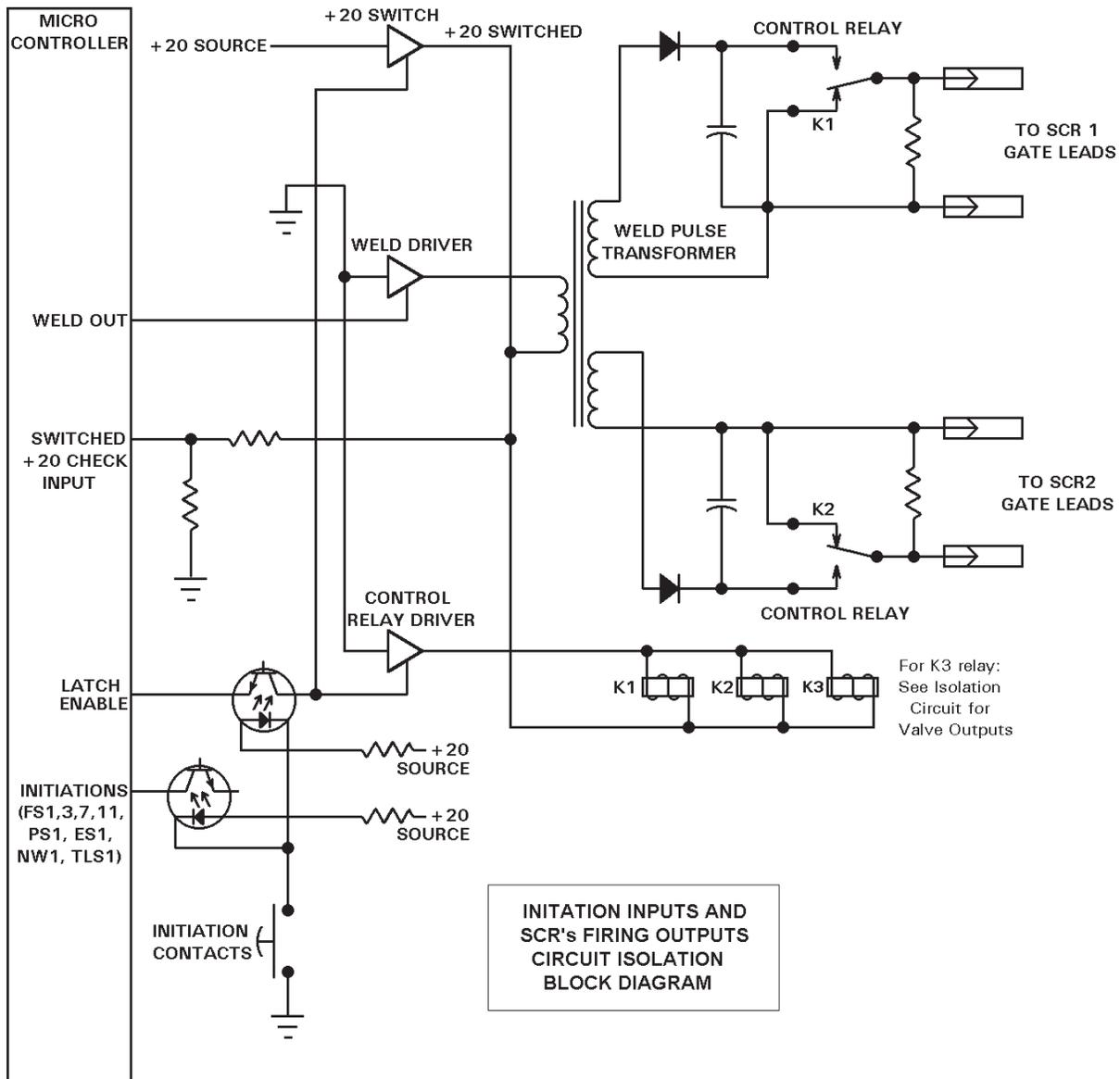
**Figure 4-14.** Isolation circuit block diagram
