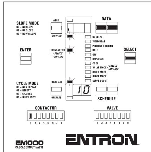
Figure B16. SELECT CONTACTOR and program 01 (Contactor 1)
