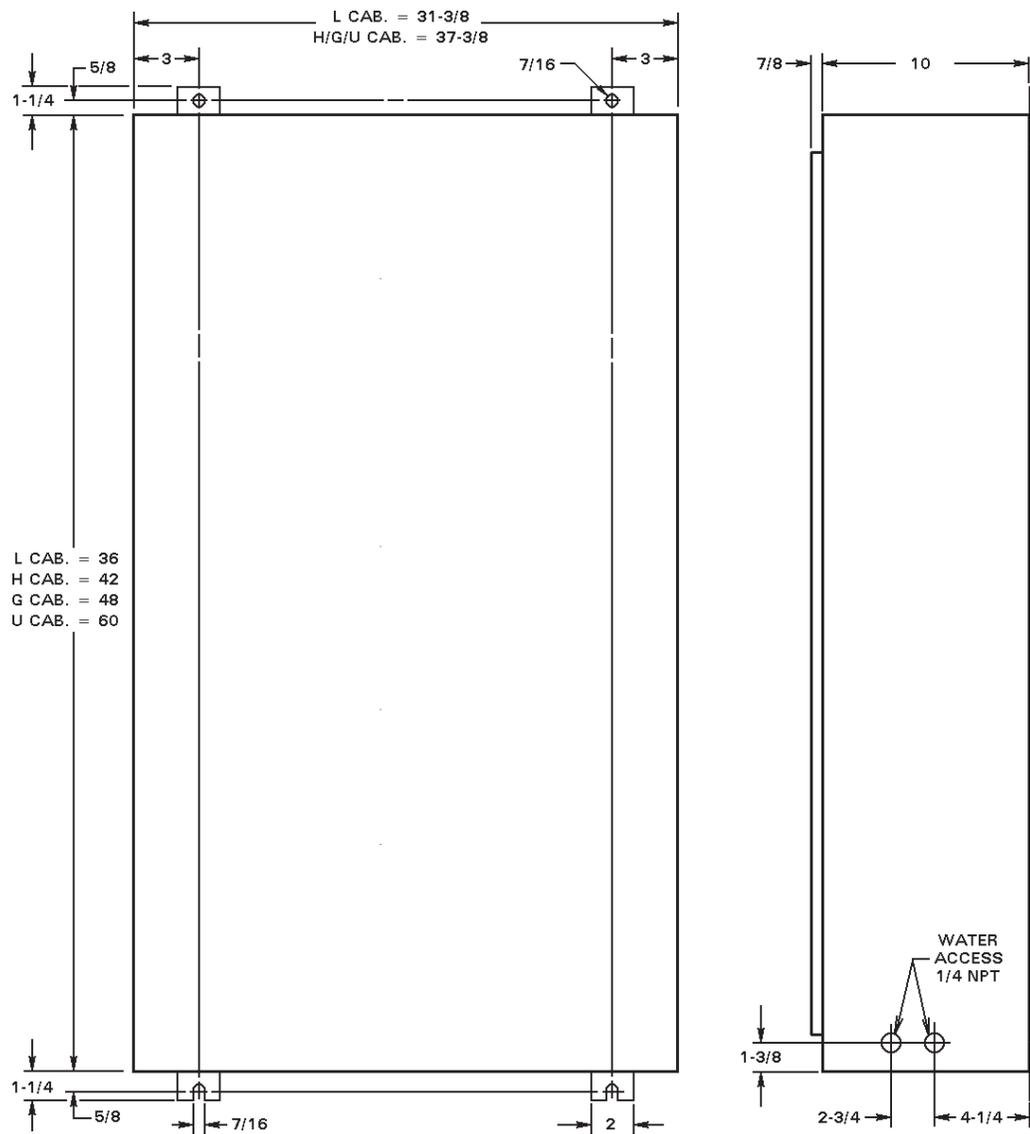
**Figure 3-2.** Mechanical mounting diagram for “L/H/G/U” cabinets
