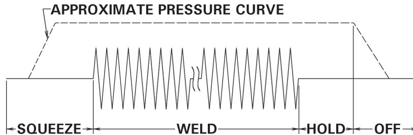
Figure 9-7. CONTINUOUS SEAM mode
