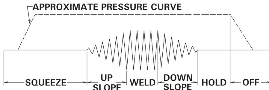
Figure 9-4. UPSLOPE and DOWNSLOPE with CHAINED mode
