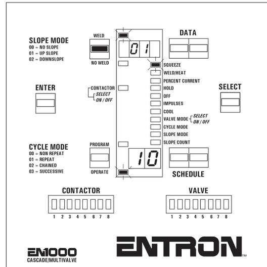
**Figure B19.** *Put control in WELD mode*
