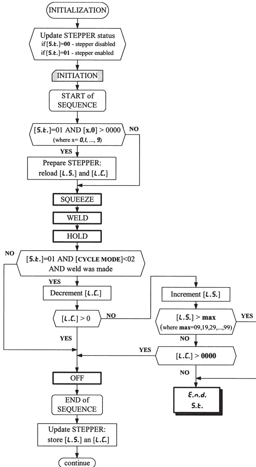
Figure 7-6. Stepper Operation Algorithm
