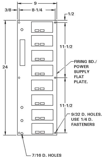
**Figure 3-4.** *Firing Board Assembly mounting detail*
