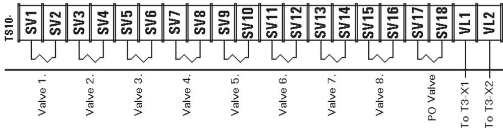
**Figure 6-4.** Terminal Strip TS10 valve outputs
