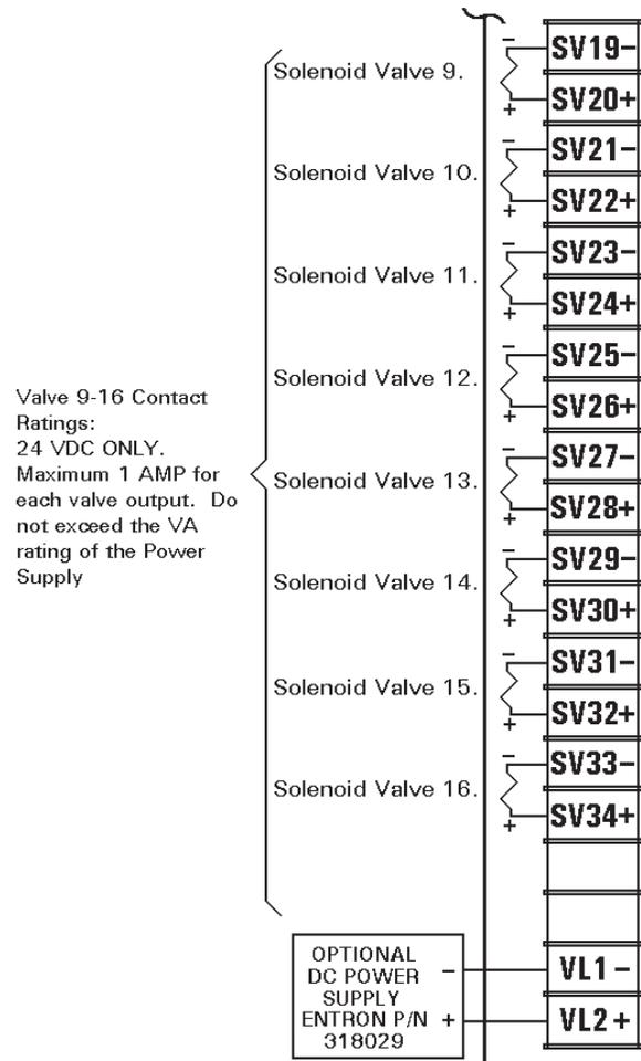
VALVE OUTPUT BOARD ASSEM. NO.
