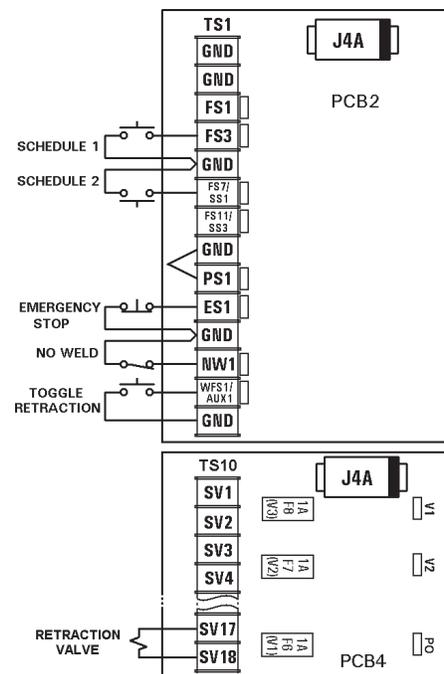
**Figure 9-11. Momentary Retraction connections**
