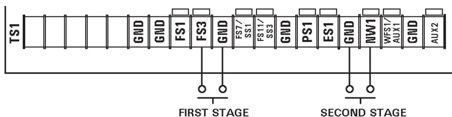
**Figure 9-9.** Using Two Stage initiation in BRAZING mode
