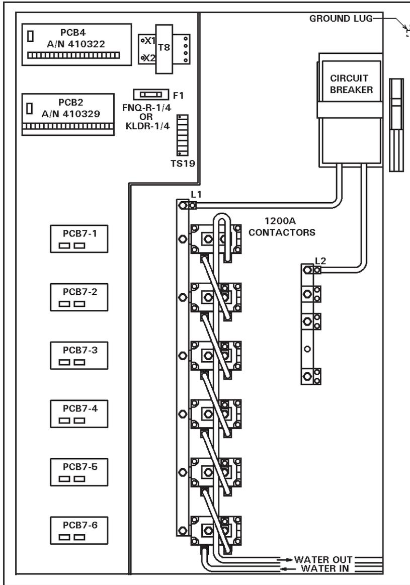
**Figure 3-1.** Style “G” Cabinet – 1200A Contactors
