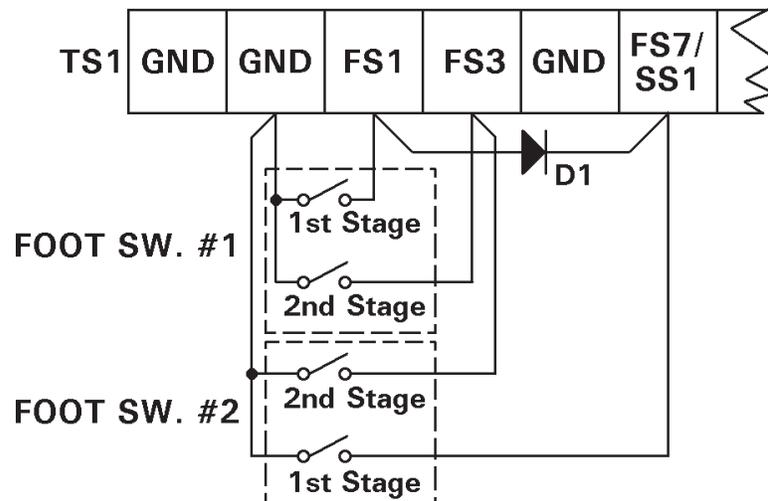
**Figure 5-11.** Dual two-stage foot switch initiation
