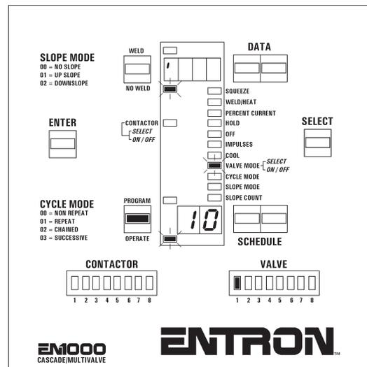
Figure B17. Put control in OPERATE mode
