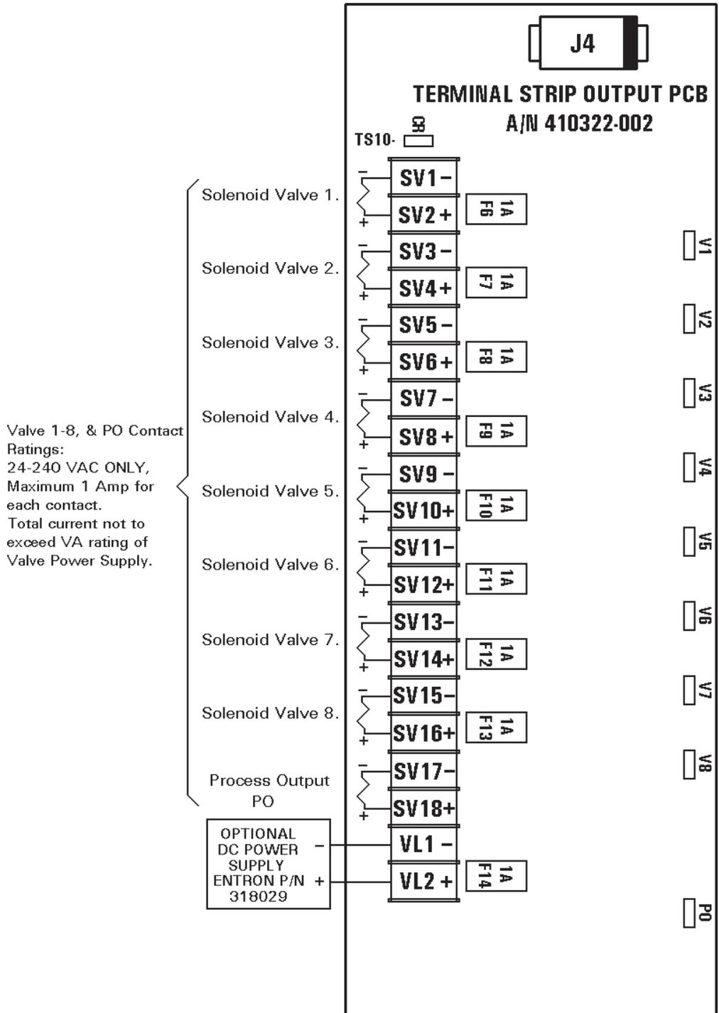
**Figure 4-7.** Terminal Strip Output Board for 24 VDC
