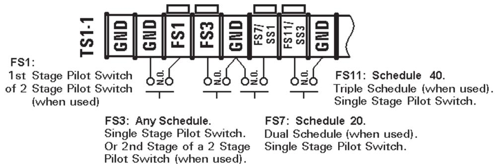
**Figure 4-8.** *Initiation inputs on Terminal Strip TS1*
