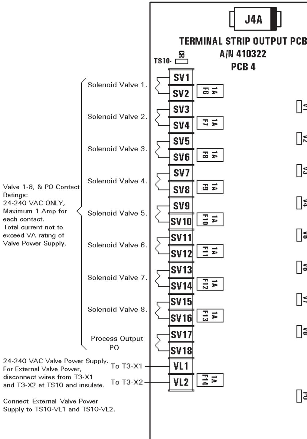
**Figure 4-6. Terminal Strip Output Board for 24-240 VAC**
