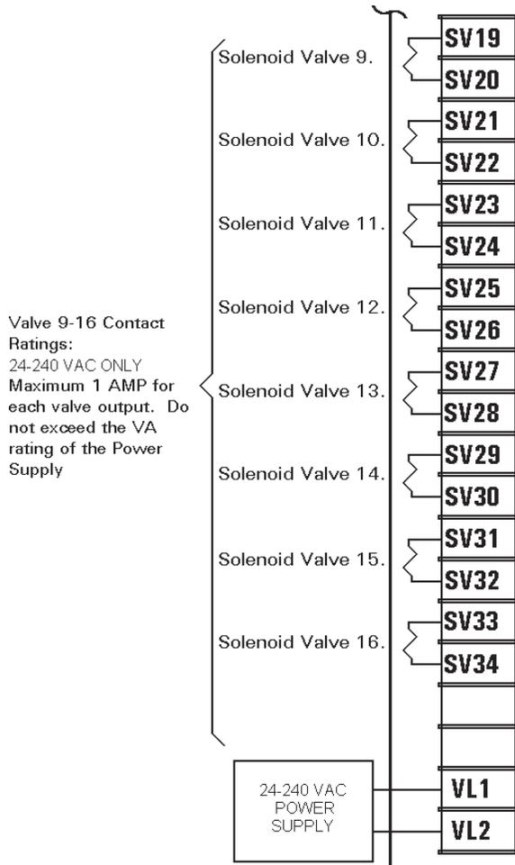
VALVE OUTPUT BOARD ASSEM. NO.
